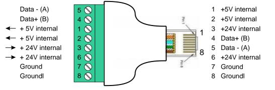
The adapter is available for standard-wiring as accessory.
