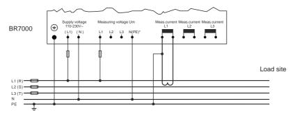
Alternative 3: single-phase measuring as alternative 2, but with capacitor current measuring in the compensation system for collection of real capacitor currents.
