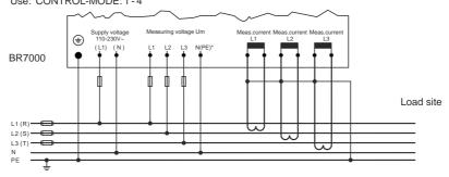
Alternative 2: single-phase measuring via current transformer in L1 Values extrapolated (balance assumed).
