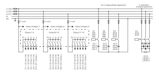
In case of the setting the BR7000 will automatically assign the capacitors according to the wiring diagram.
