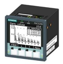
SENTRON, meas. device & power quality recorder, 7KM PAC5200, LCD, L-L: 690 V, L-N: 400 V, 10 A, 3-phase, Modbus TCP, apparent/active/reactive energy / cos phi, harmonics: 2.-40., THD, class 0.5 acc. to IEC61557-12 or cl. 0.5S acc. to IEC62053-22, wide-range pwr sup. unit AC/DC, screw terminals
