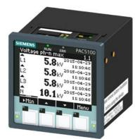
SENTRON, measuring device, 7KM PAC5100, LCD, L-L: 690 V, L-N: 400 V, 10 A, 3-phase, Modbus TCP, apparent/active/ reactive energy / cos phi, harmonics: 2. - 40., THD, class 0.5 acc to IEC61557- 12 or cl. 0.5S acc. to IEC62053-22, wide-range pwr sup. unit AC/DC, screw terminals
